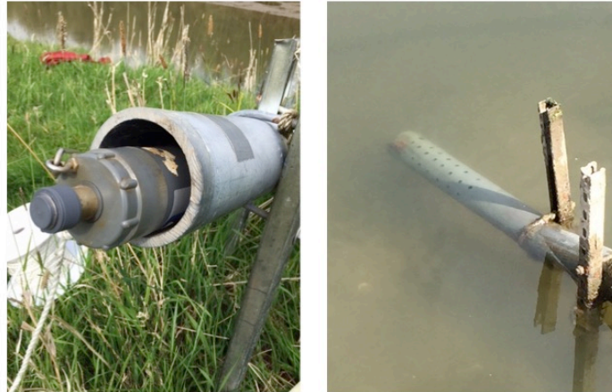
Figure 5. Images are showing deployment of water quality monitors (YSI sondes) at study sites.
